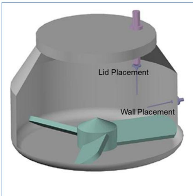
Consistent placement in the granulator across the batches that are being compared with respect to the height from the impeller and the radial distance ratio from the shaft are important parameters for consistent
