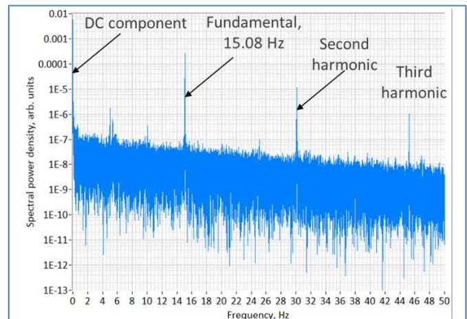
The blade frequency of 15.08 Hz gives the time interval between two blades of 0.066 seconds.
