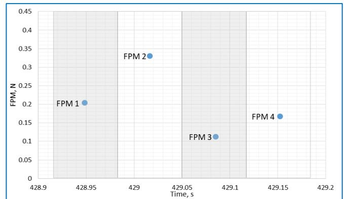
Being a differential measurement, FPM provides a reliable characteristic of the wet mass consistency and densification since it is independent from possible zero drift in the raw signal.
